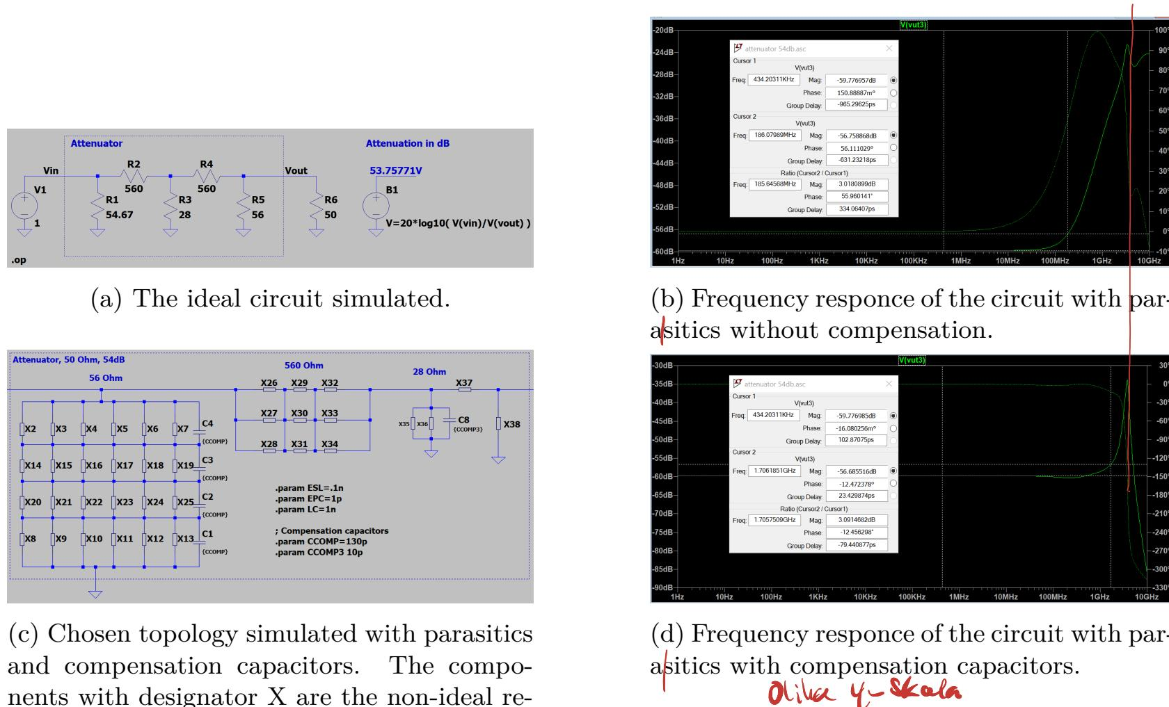
Figure 4.5: The  $50\Omega$  attenuator simulated.
