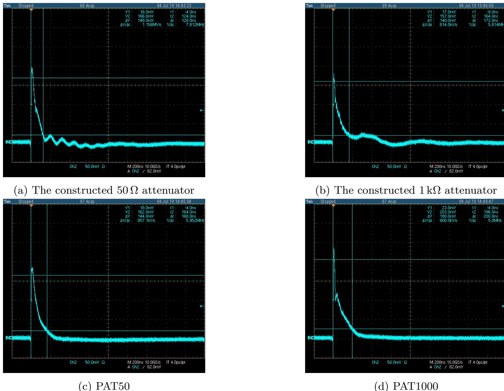
Figure 4.12: The attenuator measurements in time domain, measured with the oscilloscope.
