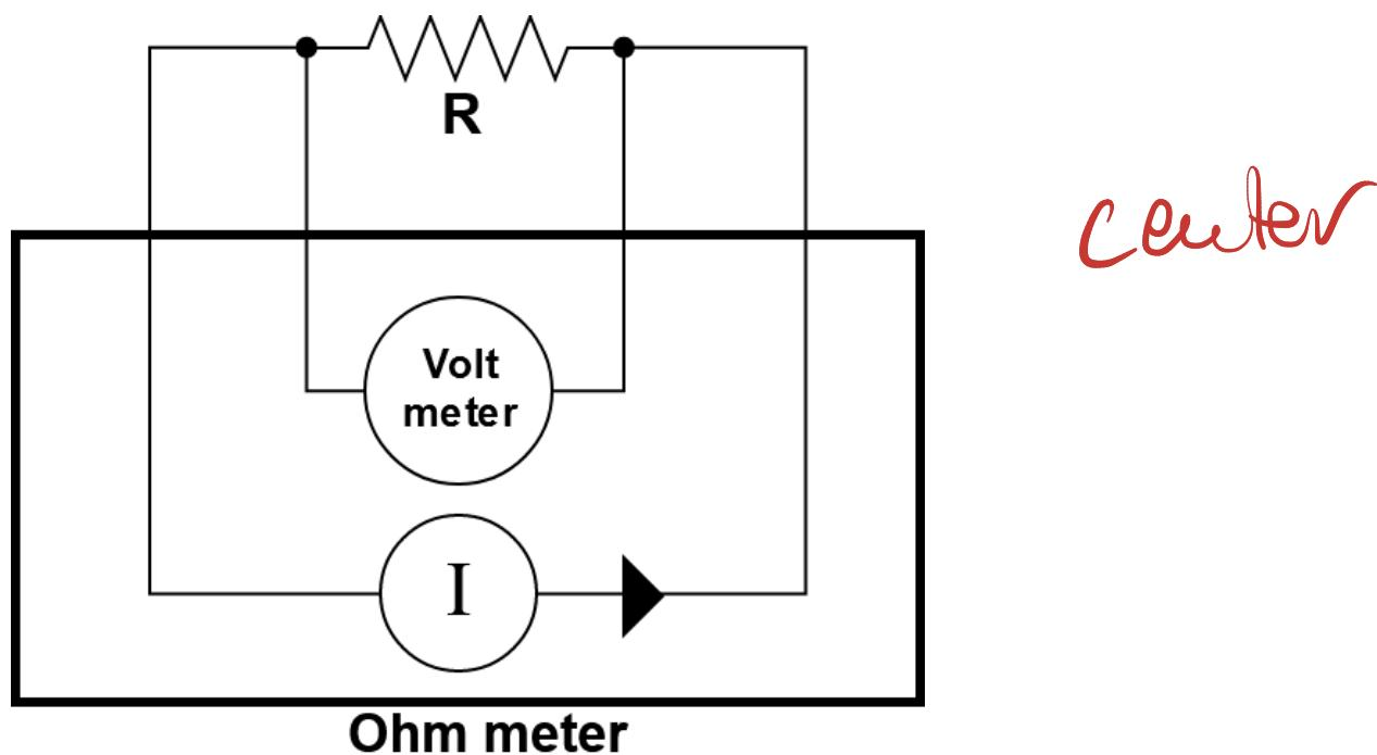
Figure 2.8: When measuring a low value resistor, the *Kelvin connection* can be used to determine the resistance at the point where the voltmeter is connected without the resistance in the probe leads affecting the result.
