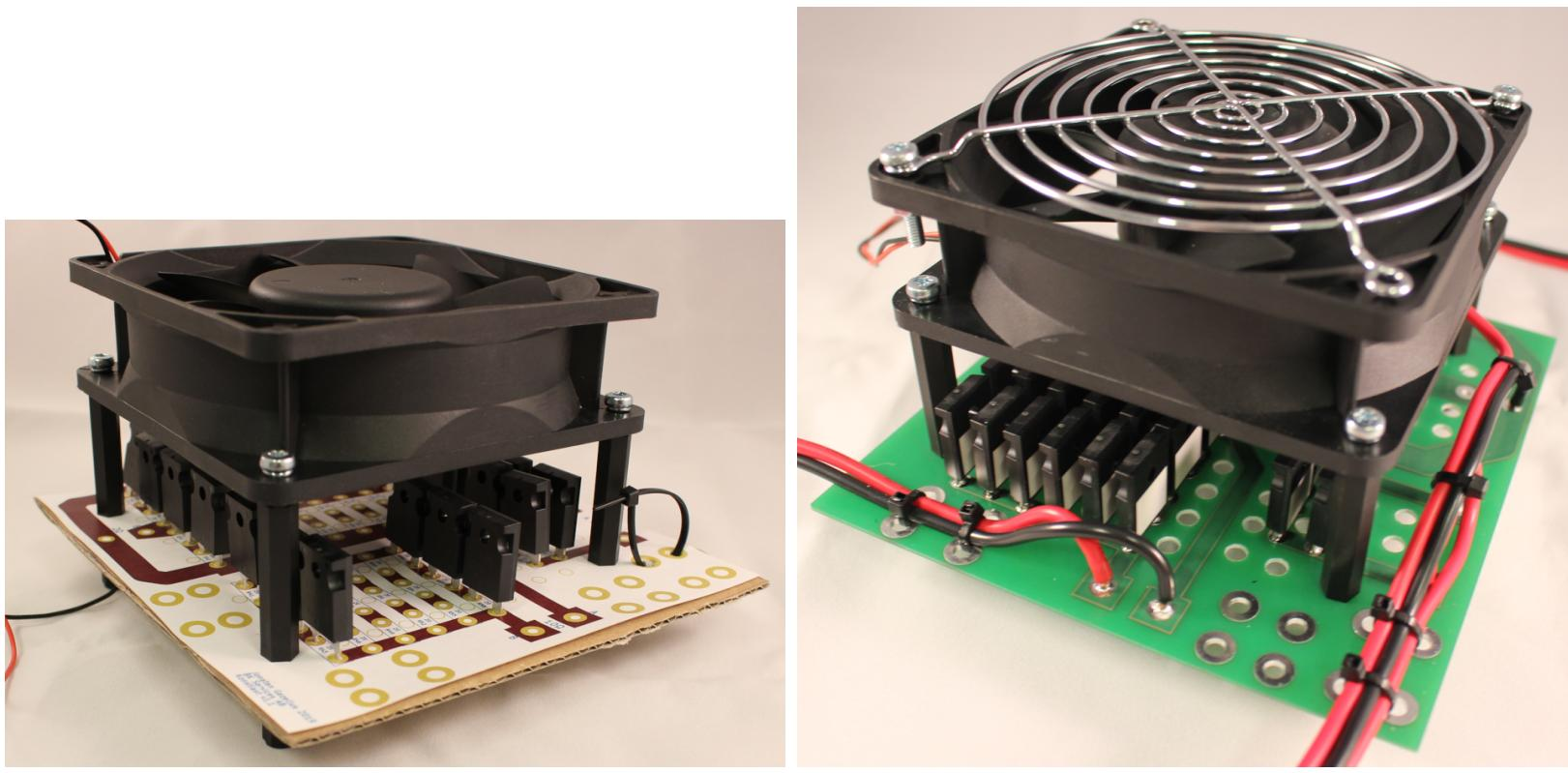
(a) Card board was used to test the PCB layout before it was sent for manufacturing.
