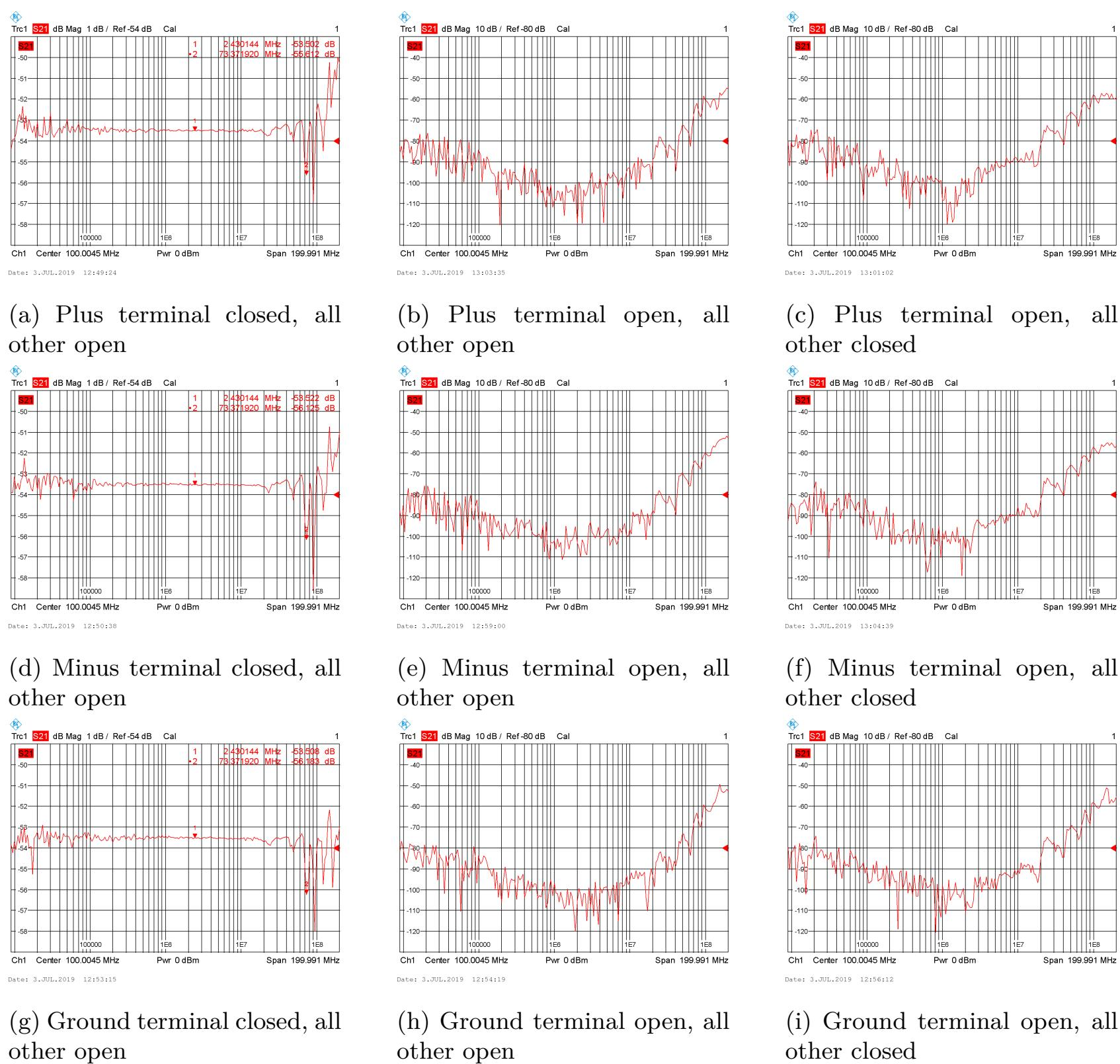
Figure 4.9: The S21 measurements for the  $50\Omega$  attenuators. No compensation capacitors have been used.
