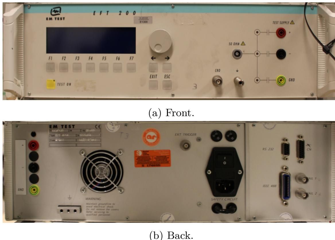
Figure 2.10: The EFT 200 is used to generate test pulse 3a and 3b.
