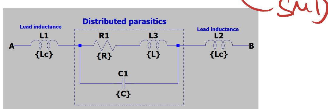
Figure 2.7: At high frequencies a resistors parasitic inductance and capacitance will affect the behavior of the circuit. This is the model used in this thesis when simulating circuits.
