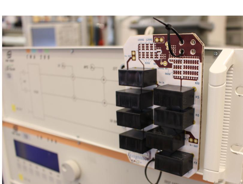
(a) Card board was used to test the PCB layout before it was sent for manufacturing.
