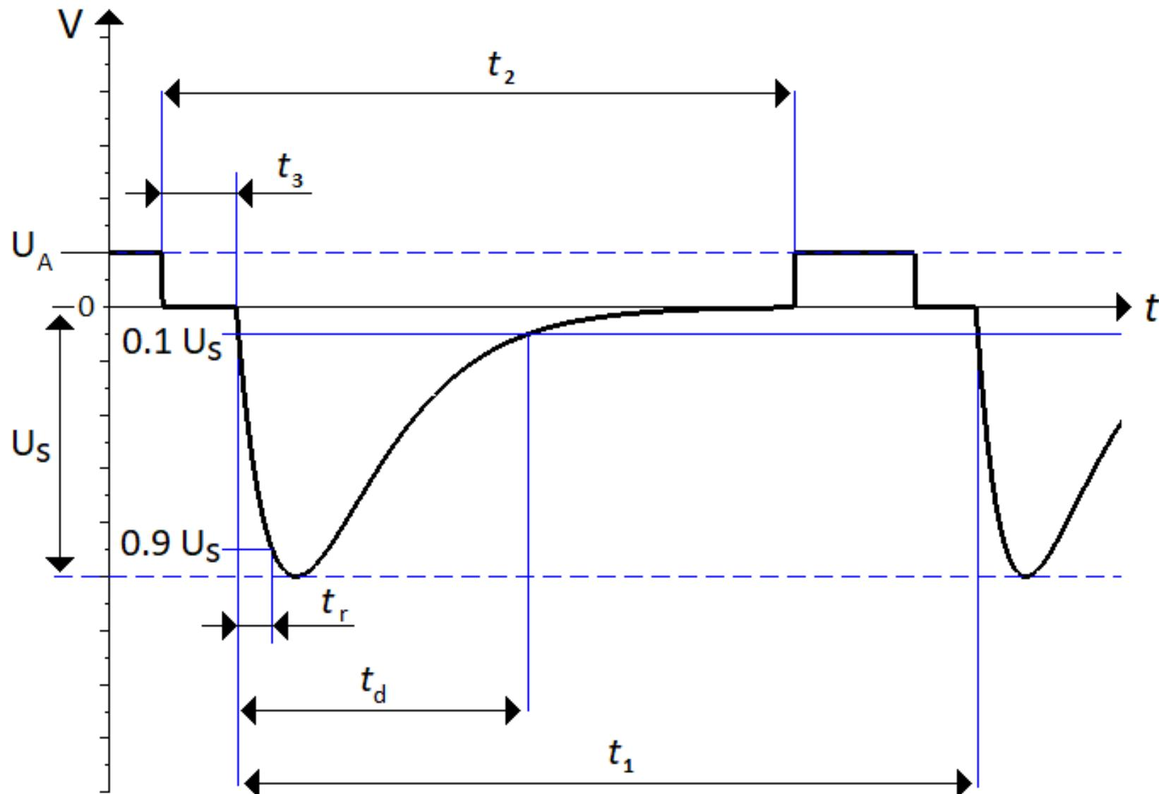
Figure 2.2: Illustration of test pulse 1.
