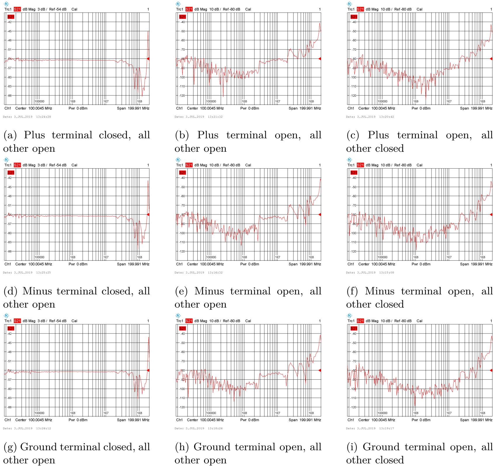
Figure 4.10: The S21 measurements for the  $1\text{k}\Omega$  attenuators. No compensation capacitors have been used.
