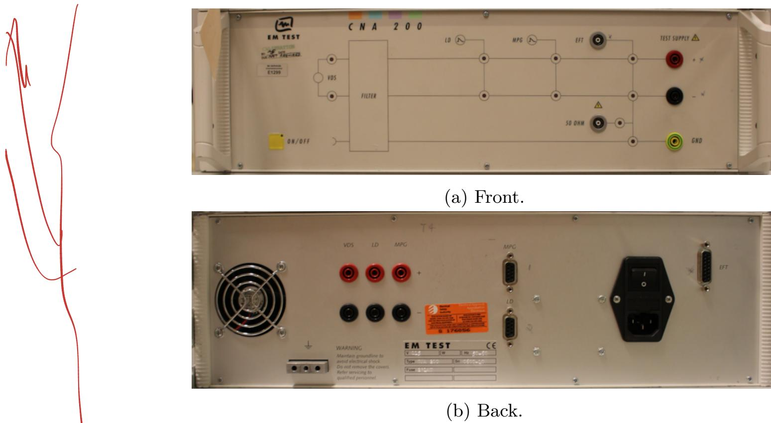
Figure 2.13: The CNA 200 is used to couple all of the other pulse generators outputs to a common output.
