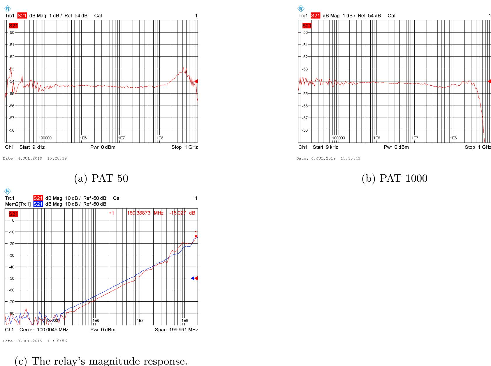
Figure 4.11: The S21 measurements on the commercial attenuators and the solo relay.
