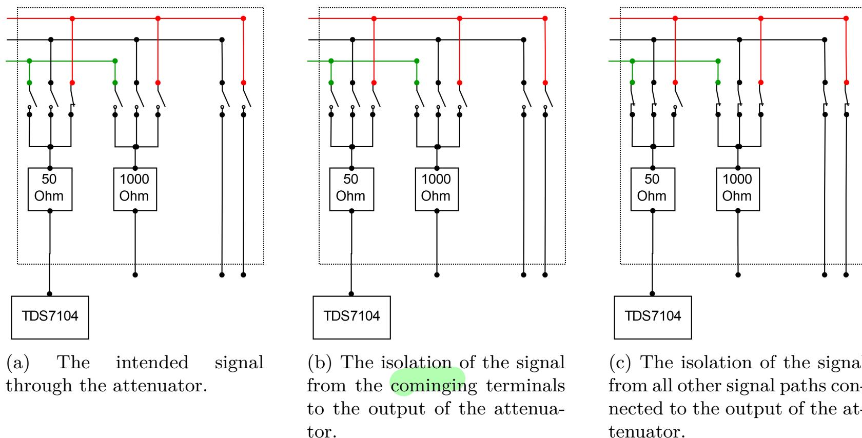
Figure 3.10: The different scenarios that were measured in frequency domain for the + terminal to the  $50\Omega$  attenuator. Corresponding measurements were made for the - and the PE terminal as well as for the  $1000\Omega$  attenuator.
