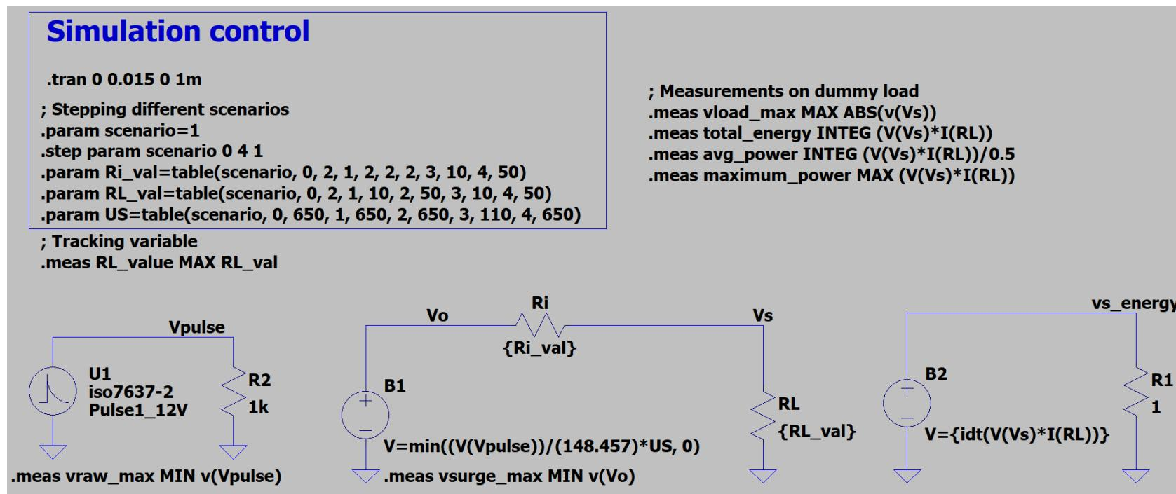
Figure 3.6: The energy transferred to the dummy load was simulated using the above LTSpice circuit for pulse 1. Similar circuits were used for the other pulses.
