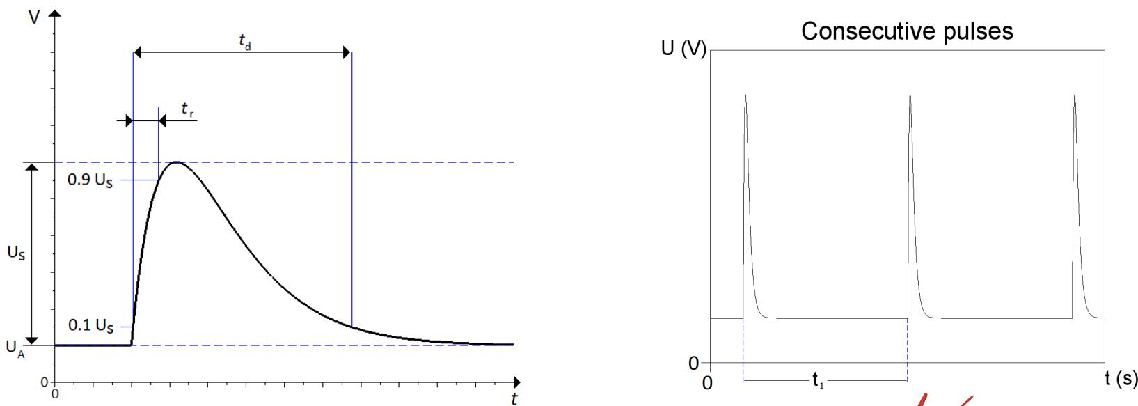
(a) The surge voltage  $U_s$  is the pulse maximum voltage disregarding the offset voltage  $U_A$ . The rise  $t_r$  time is defined as the time elapsed from 0.1 to 0.9 times the surge voltage on the rising edge of the pulse. The duration  $t_d$  is defined as the time from 0.1 times the maximum voltage on the rising edge, back to the same level of the falling edge.
