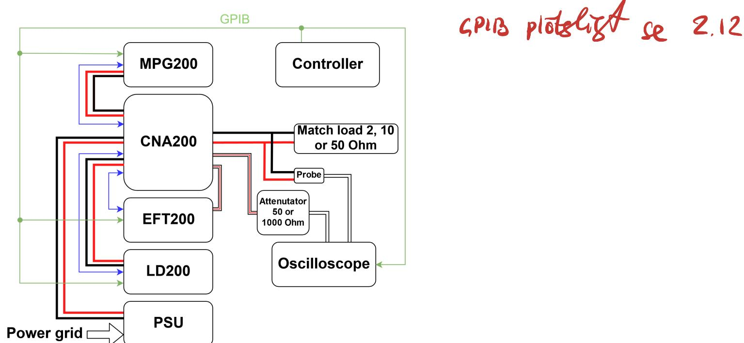
Figure 3.3: The proposed setup for alternative must be connected in different ways by a human during the verification process.
