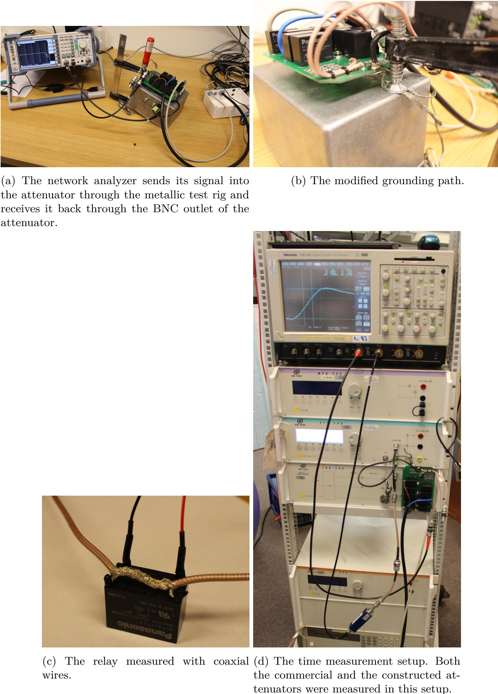
Figure 3.9: The test setups for frequency and time measurements of the attenuators.
