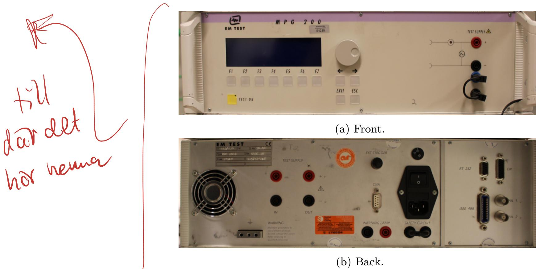
Figure 2.9: The MPG 200 is used to generate test pulse 1 and 2a.
