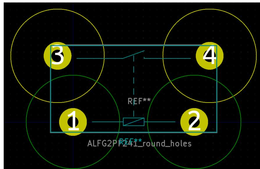
Figure 3.8: Decorational circles were made on the relay footprint to mark the creepage and clearance distance required. *dimensions &c*
