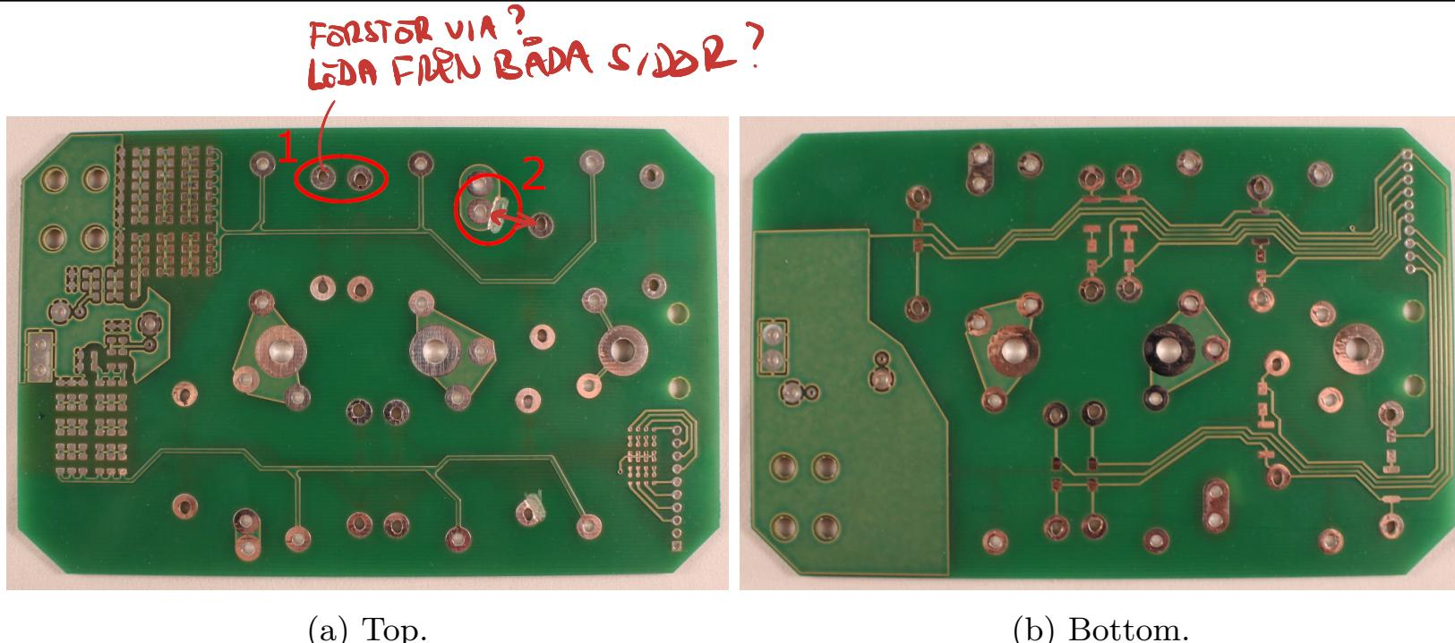
Figure 4.8: The PCB was modified to correct the mistakes. The footprint for the relay was slightly wrong (1) and some of the creepage distances were to short (2)
